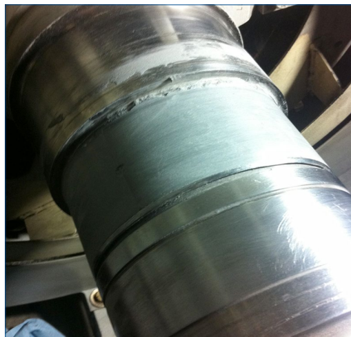
The repaired shaft after
